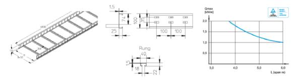
The cable ladder is made of steel 1.0122 and after fabrication galvanised according to ISO 1461. The cable ladder is designed and constructed to use as a support system for electrical and instrument cables. Use by other disciplines is not allowed.
