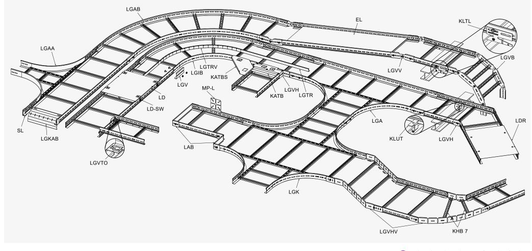
Please always observe the support distance in conjunction with the load-bearing capacity of the cable ladders and the correct choice of dowels!
