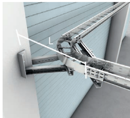
5 | Horizontal Heavy-duty corner installation (EBW) for horizontal 90° bends with side rail support (WPHS-K) has to be mounted on a concrete support. L = width of wide-span cable ladder + 560 mm
